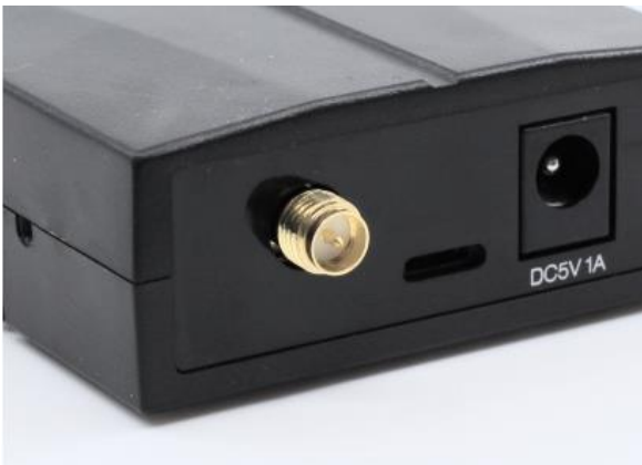
Figure 1-6 RP-SMA jack for an antenna
