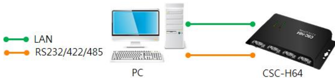
Figure 2-8 connection between CSC-H64 and a PC
