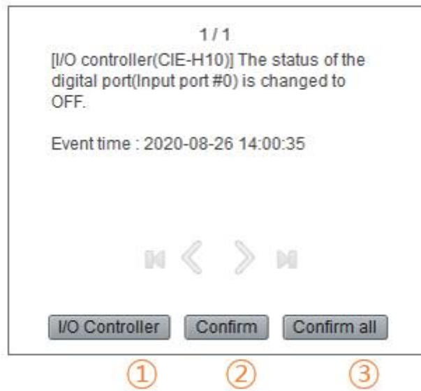
Figure 2-52 Notification message box
